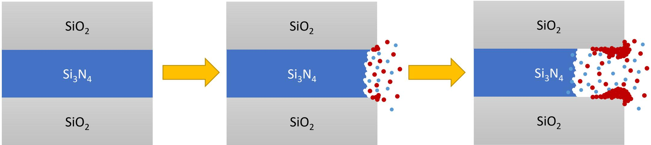
By-products (red circles) during Si<sub>3</sub>N<sub>4</sub> (blue circles) etching
