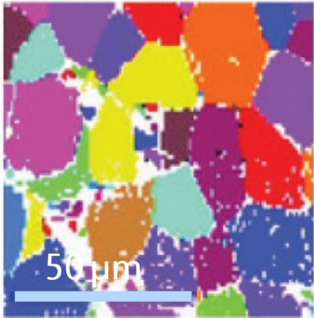
Electron backscattering diffraction plot for halide perovskite E Tennyson et al Nature Rev Mater (2019)
