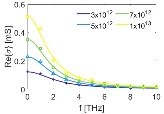
Fig. 2. Real part of  $\sigma(\omega)$  as a function of terahertz frequency for different electron densities in suspended monolayer MoS<sub>2</sub>. The impurity density throughout is  $10^{12} \text{ cm}^{-2}$ . The points are numerically calculated and the solid lines are Drude fits.
