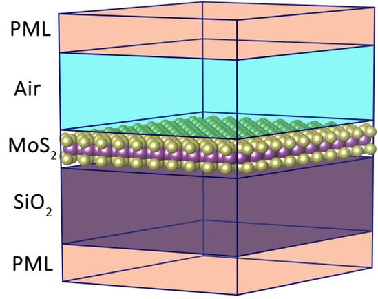
Fig. 1. Schematic of the three-dimensional (3D) simulation geometry of monolayer MoS<sub>2</sub> between air on top and SiO<sub>2</sub> substrate on bottom. The vertical boundaries have periodic boundary conditions.
