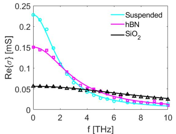
Fig. 3. Real part of  $\sigma(\omega)$  versus frequency for MoS<sub>2</sub> that is suspended, supported on hBN, and supported on SiO<sub>2</sub>.
